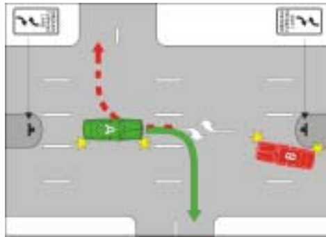
Giving way in a median turning bay
